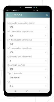
The application gives us the possibility to calculate: symmetrical and asymmetrical cuts of the netting panels, codend design, calculate lengths of the sweeps sections, designs with square mesh, diamonds, netting weight, twine area, filtration ( $U_1$  and  $U_2$ ) and netting area.
